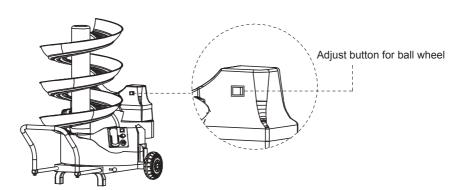
Special attention: Adjust button to adjust the distance between the two shooting wheel; Wide distance makes weaker speed, narrow distance makes higher speed.
